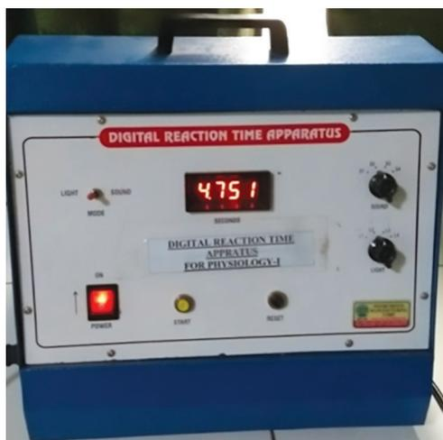
Fig. 1: Digital reaction time apparatus operator (investigator) side
